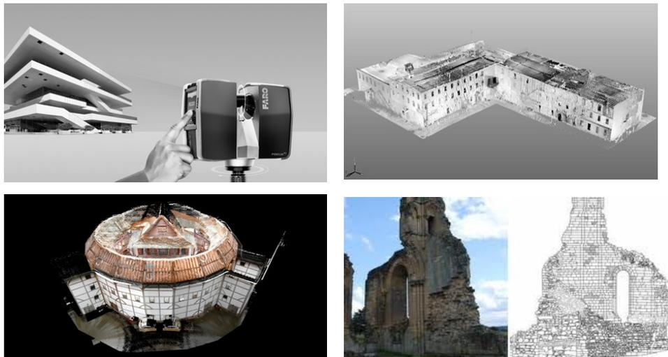
Figure 5 Laser scanner and scanned models [7].
